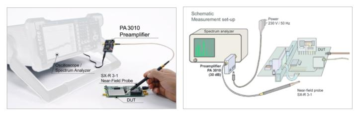
Figure 6 - Measurement set-up with PA 3010, spectrum analyzer, near-field probe and DUT
